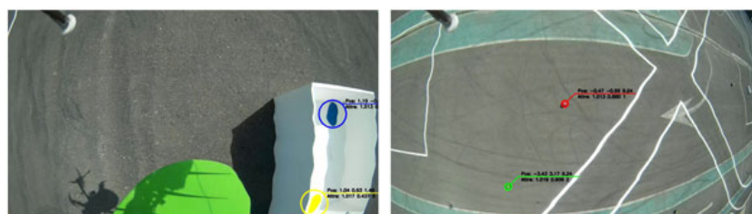
FIGURE 3 Object detection in onboard camera images affected by the 'jelly' or 'wobble' effect, which deforms lines (left image), as well as circular and square objects (right image). The detection results indicate the 3D relative position (top line) and attributes like roundness, eccentricity and type (1,2,3 for red, green, and blue static objects and 5 for the yellow moving object) [Color figure can be viewed at wileyonlinelibrary.com ]
