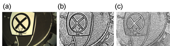
FIGURE 4 (a) Image taken by the camera, (b) result of the adaptive threshold with box size of 11 pixels, and (c) adaptive threshold with box size 5 pixels. The box size is variable and depends on the thickness of the expected segments in the landing pattern and decreases with the height of the unmanned aerial vehicle [Color figure can be viewed at wileyonlinelibrary.com]
