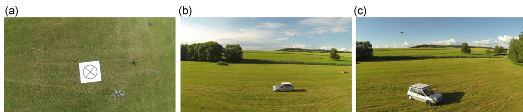
FIGURE 12 Photos from the first experiments in the field. (a) a UAV hovering above a static target, (b) a UAV tracking a vehicle moving along a linear trajectory, and (c) first attempts with tracking a ground vehicle moving in circles. The linear Kalman filter was used to estimate the states of the ground vehicle during this stage of development. Additional video material documenting these experiments can be found at http://mrs.felk.cvut.cz/jfr2018landing-video1 . UAV: unmanned aerial vehicle [Color figure can be viewed at wileyonlinelibrary.com]
