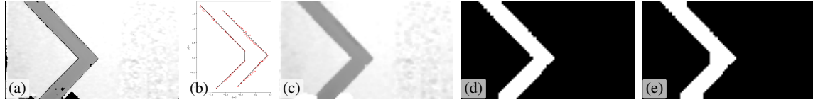
Figure 9: Original depth data (a) used for computing the result of the wall detection (b). The depth data are first filtered to lower resolution (c), then thresholded using wall height (d), and applied with the morphological closing operation (e).
