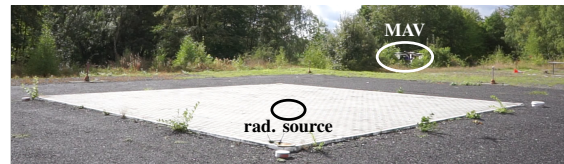
Fig. 10: Photo of the autonomous MAV while mapping the radiation environment using the Timepix detector.
