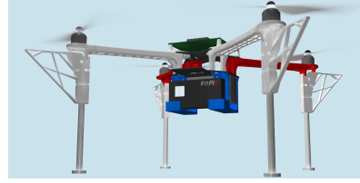
Fig. 7: The DJI F450 quadrotor with a FITPix device mounted to the front of the frame. The 14 \times 14 mm Silicon surface of the Timepix detector is visible as a silver square.
