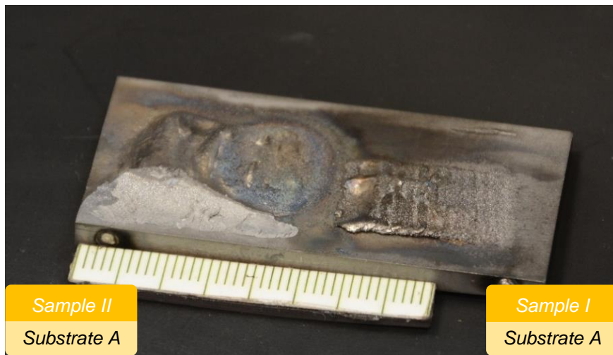
Figure 8.1: Photograph of substrate A with deposited Samples I (right) and II (left)
