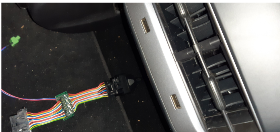
Figure 3.3: Rear USB ports and OBD-II connector
