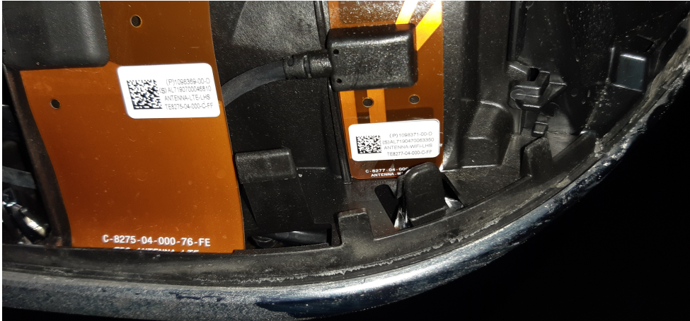
Figure 3.4: Disassembled left mirror with Wi-Fi and LTE antenna
