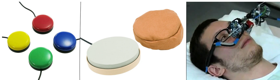
Figure 2.8: Tools for individuals with motor impairments: orby switches, pillow switches, eye tracking device. Borrowed from [22] [23] [24]
