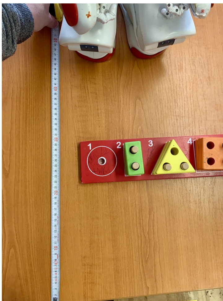
Figure 4.4: Nao standing 45 cm away from the edge of the table and the shape matching game at 21—29 cm
