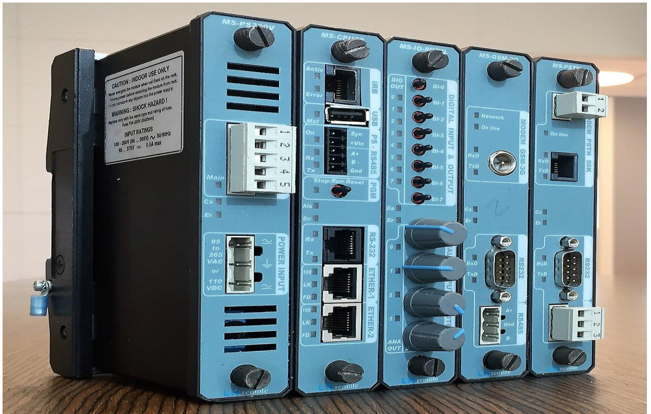
Figure 4.9 Remote Terminal Unit [21]
