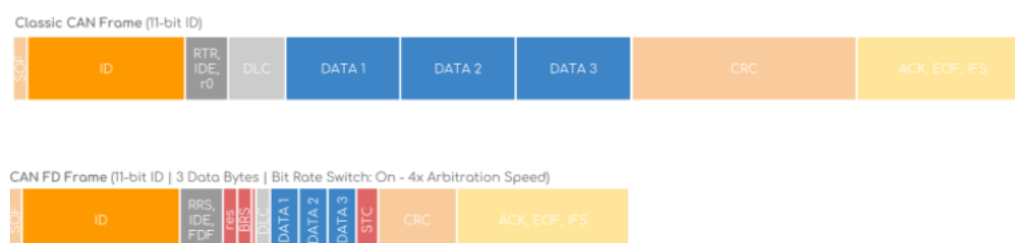
Figure 3- Classic CAN vs CAN FD –with BRS
