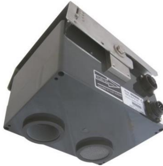
Figure 10: Example of the ASIM traffic detector
