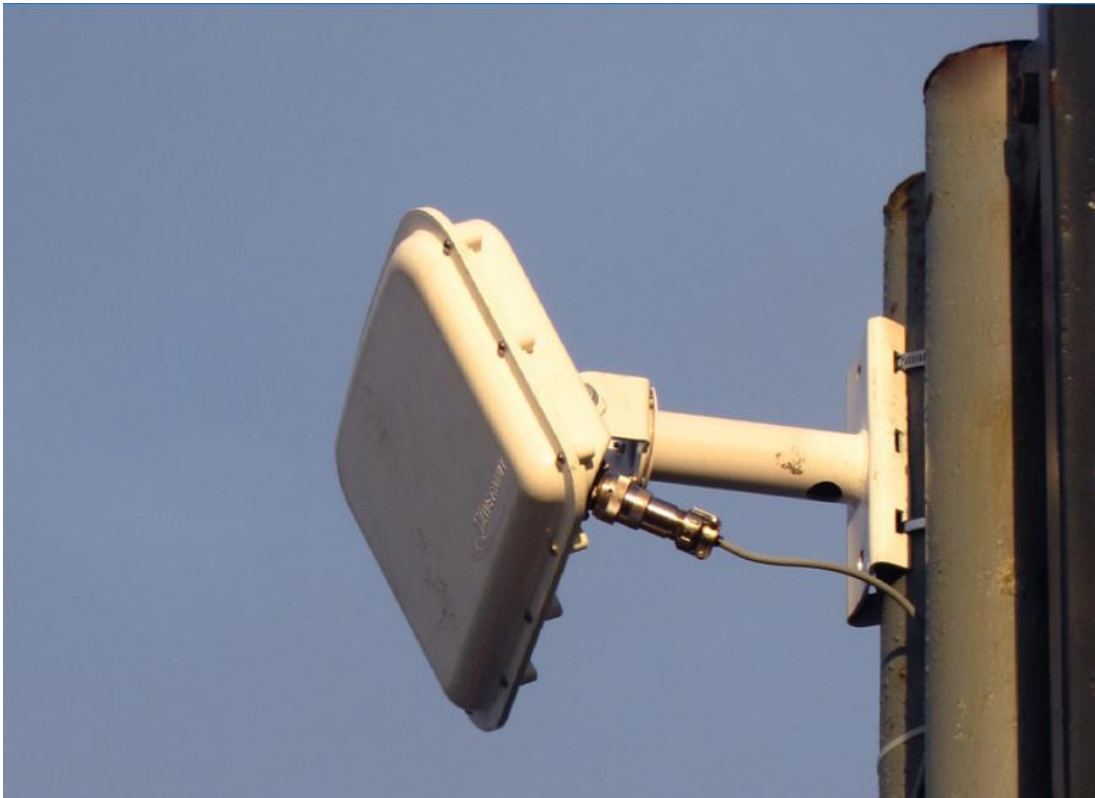
Figure 2: Example of a stationary automatic traffic counter – type Wavetronix (15)
