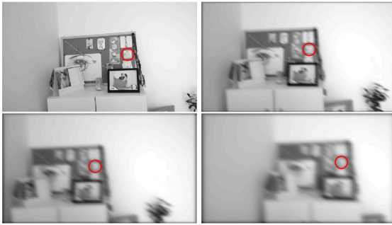
Fig. 10. Tracking in a blurred video. The initial clear image with the template (top left), sample frames of the blurred video with the template detected.
