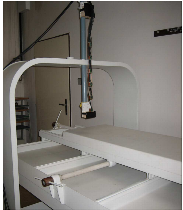
Fig. 2. Measuring magnetopneumographic bed with the gradiometer fixed into a separate portal.
