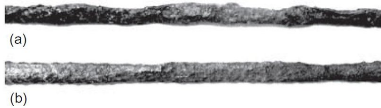
Figure 2.4: Comparison between steel rebar corroded by natural carbonation a) and artificial carbonation b) [85].
