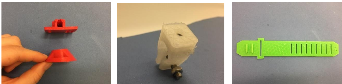
Figure 31. Synthesis I. Material selection. PLA flex picture A. Nylon picture B. TPE picture C.
