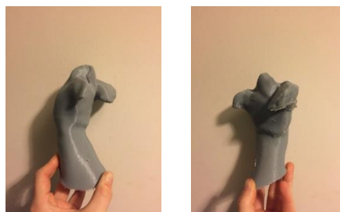
Figure 53. Hand 3D model acquisition. User' hand printed in PLA
