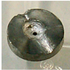
Fig. 31: Detail of our single stream nozzle after 2000 shots.
