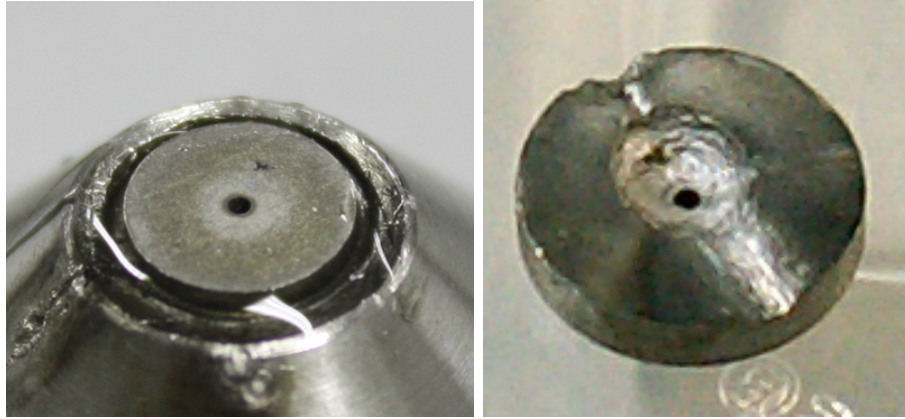
Fig. 22: Picture of the nozzle in SXR source system in XUV Laboratory at FBME, CTU in Prague. On left side new nozzle in a holder is depicted, on the right side is the detail of nozzle after 2000 shots.
