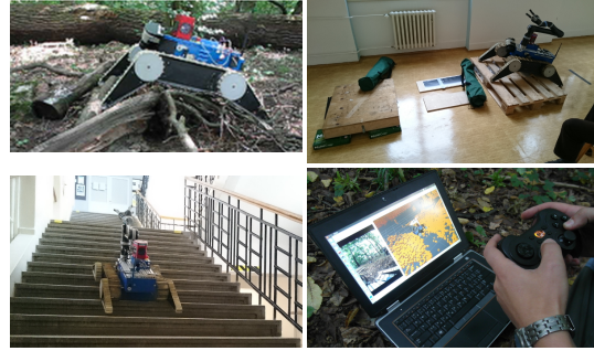
Fig. 5. Top left: Forest obstacle. Top right: Rubble obstacle. Bottom left: Stairs obstacle. Bottom right: Operator controlling the robot using only sensor data.
