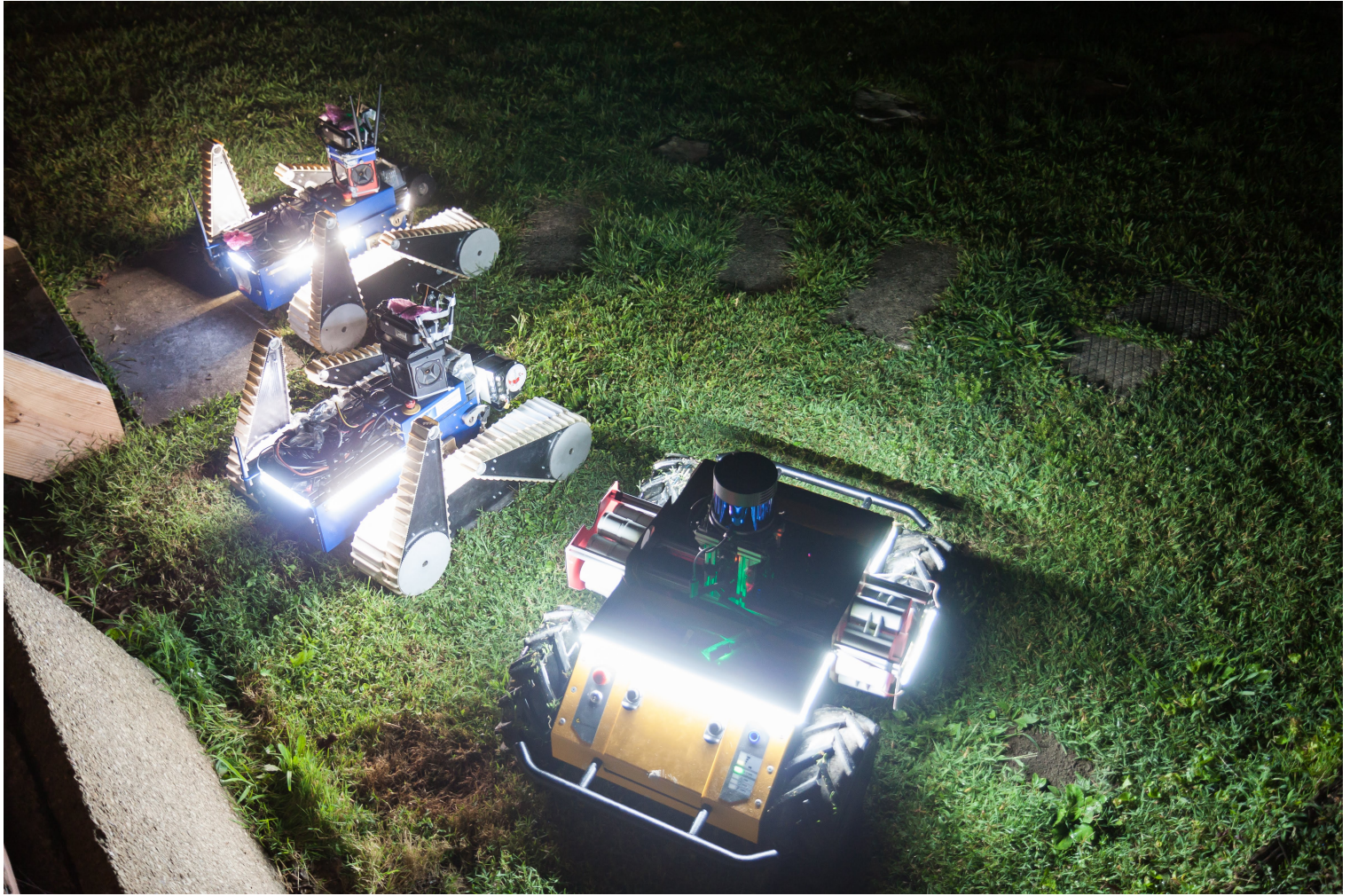
Figure B.5: SubT Challenge: The three UGVs ready to start a training mission. Strong on-body illumination is apparent in this photo, and was required in the dark parts of the tunnels in the competition.
