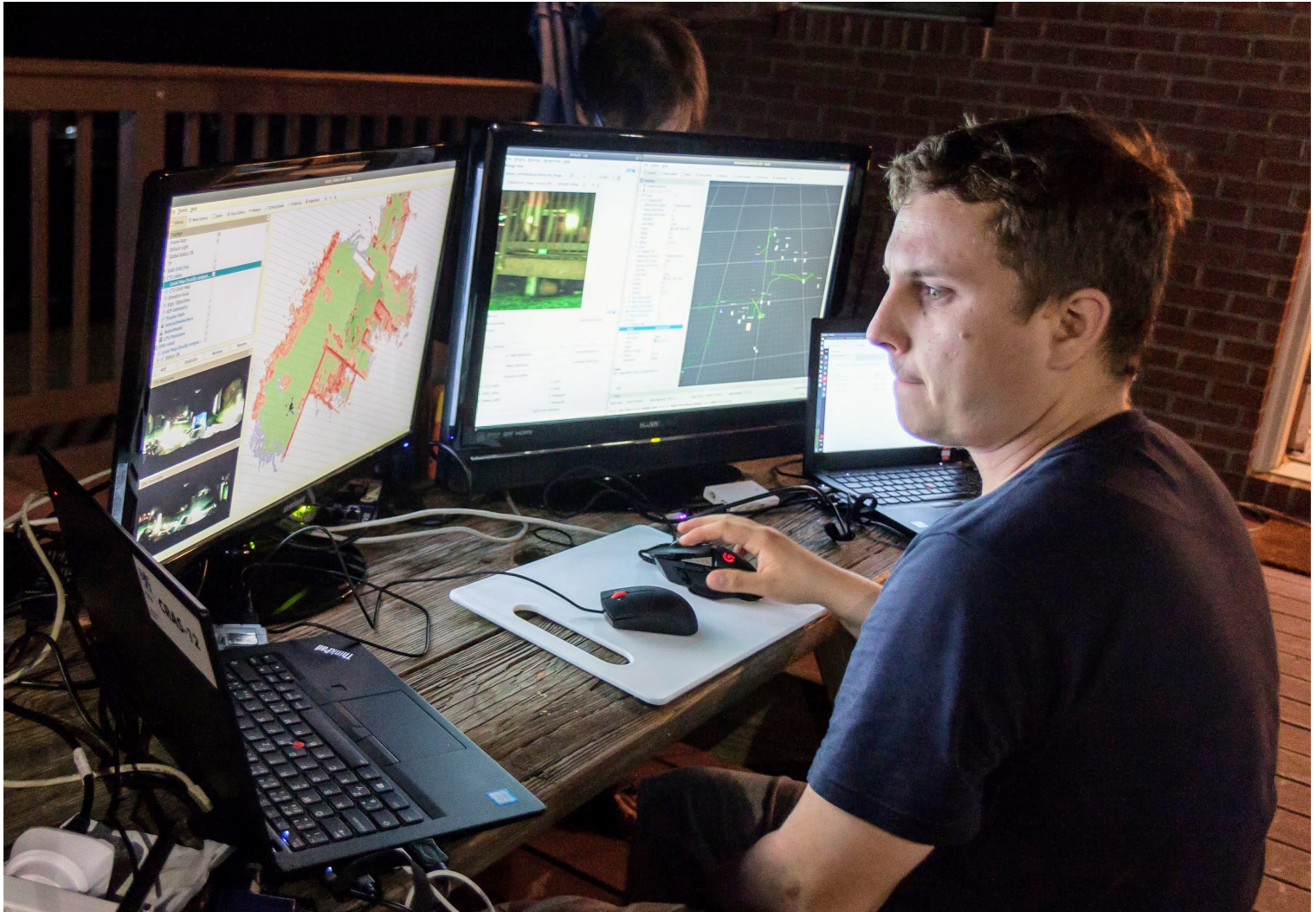
Figure B.6: SubT Challenge: Operator console showing mostly maps of the explored environment, detected artifacts, and if connection is good, also video stream from all exploring robots.
