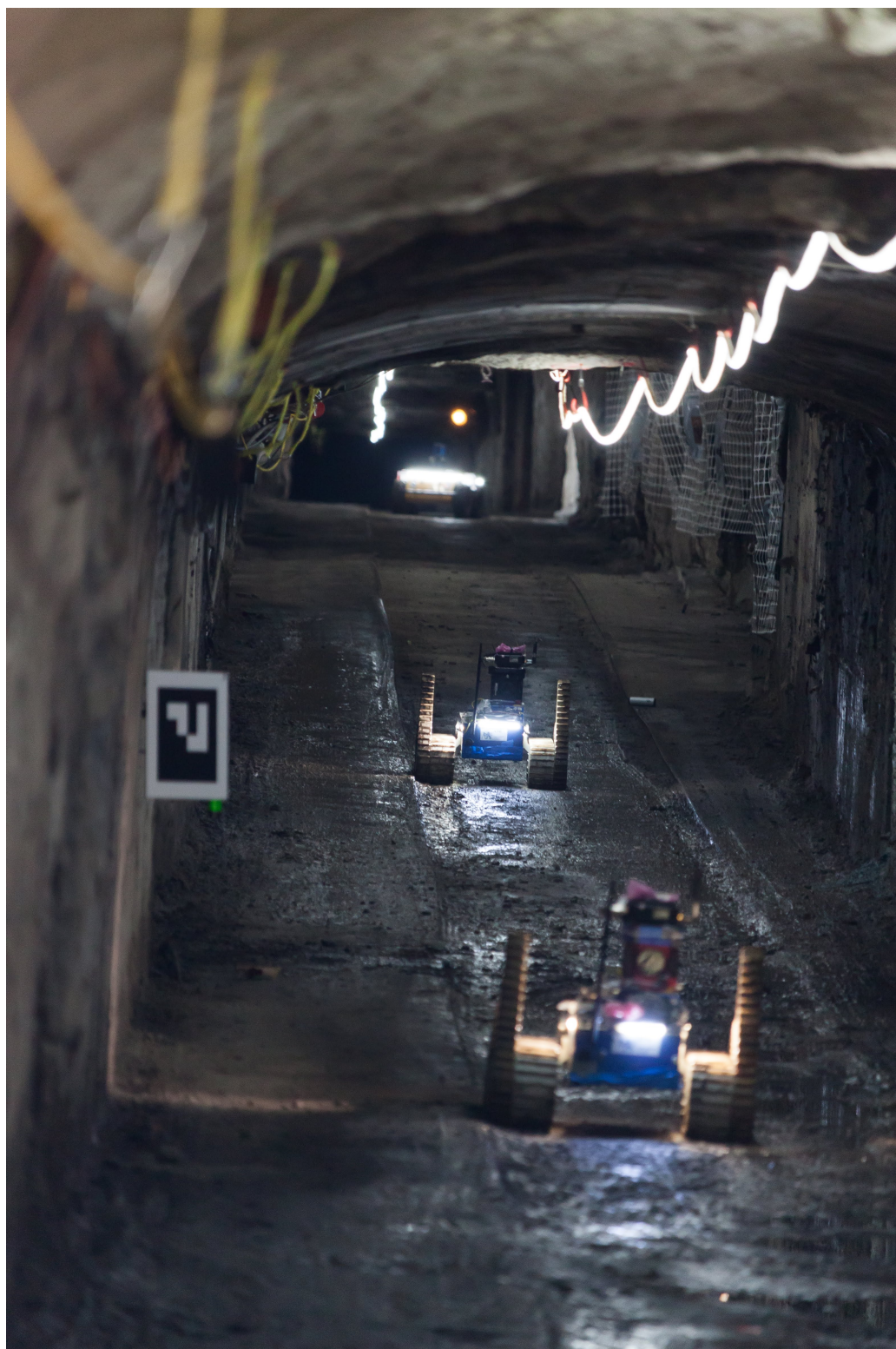
Figure B.8: SubT Challenge: Three UGVs and one UAV (hard to spot) explore the competition tunnel at the same time.
