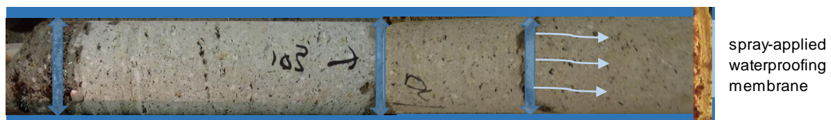
Fig. 68 Primary lining water path
