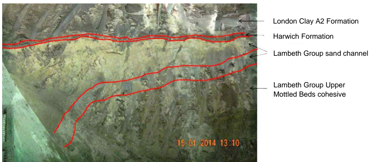
Fig. 25 Dry sand of Lambeth Group after depressurization
