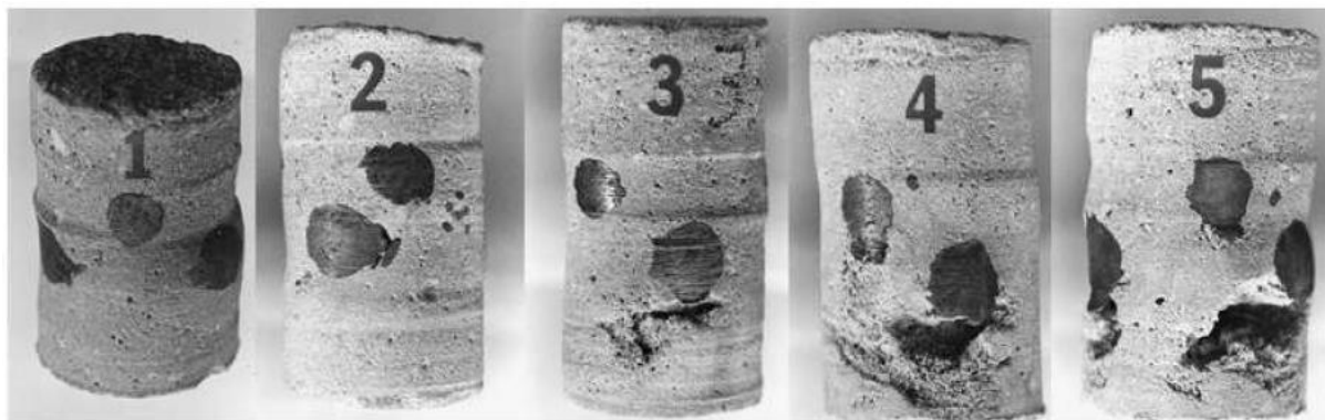
Fig. 47 Core grading according to ACI 506, [21]
