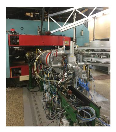
Figure 3.3: Cyclotron U-120M in the Nuclear Physics Institute of the Czech Academy of Sciences in Řež. The beamline for protons and deuterons, extracted in the negative regime, is terminated by the energy degrader unit.
