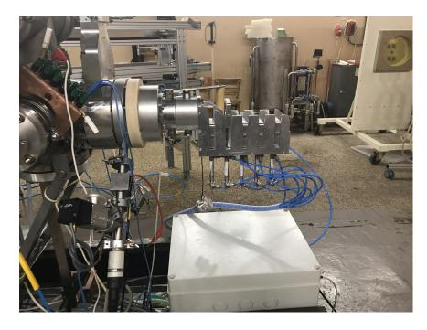
Figure 3.8: Photo of the degrader unit with aluminum plates behind the beamline exit window. During the irradiation, we used the 0.55 mm thick aluminum plate to make the beam profile wider. The initial energy of the proton beam is about 35 MeV. After passing through the degrader plate and air it reduces to  $\sim 30$  MeV at the sample position.
