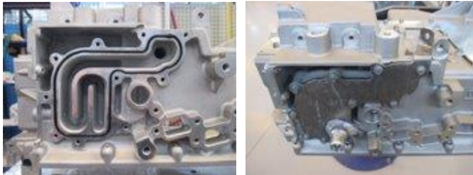
Figure 42: second part of cooling system for PEC
