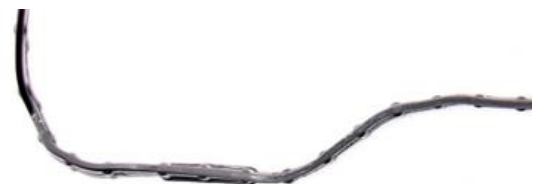
Figure 36: Fixations holes not surrounded by the gasket
