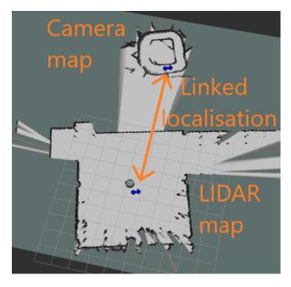
Figure 4.5: An illustration of Combined SLAM
