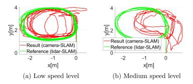
Figure 7.24: Final path estimation visualisation on the oval circuit
