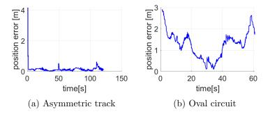
Figure 7.26: Pure localisation mode - position error at the low speed level
