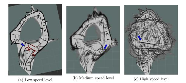
Figure 7.21: Map samples of the asymmetric circuit constructed by Global SLAM
