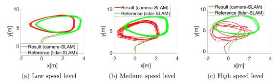
Figure 7.20: Final path the visualisation asymmetric circuit
