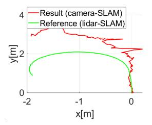
Figure 7.17: 2D LIDAR-like scanning of images - the estimated path on the oval circuit compared to the reference
