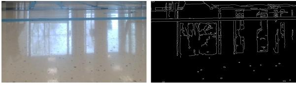
(a) The original image (b) The edge detection result
