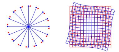
Figure 2.10: Tangential distortion illustration (from [42]; the original points are highlighted in red, the distorted points in blue)
