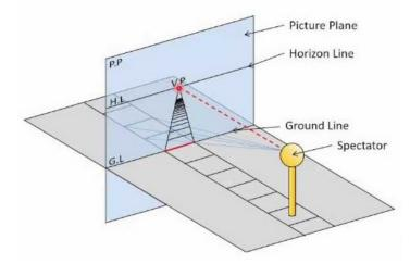
Figure 2.6: Perspective view of a plane illustration (from [12])
