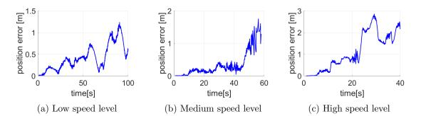
Figure 7.2: Position estimation error on the asymmetric circuit
