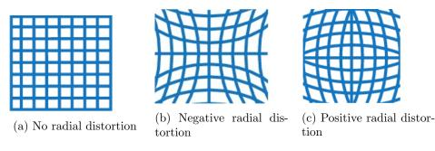
Figure 2.9: Radial distortion illustration (from [37])
