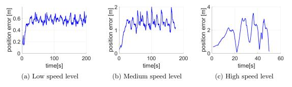
Figure 7.18: Global SLAM - position error on the asymmetric circuit
