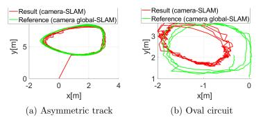
Figure 7.28: A path visualisation on the asymmetric circuit
