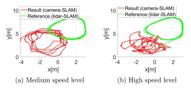
Figure 7.30: Pure localisation mode - path comparison on the asymmetric circuit
