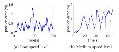
Figure 7.22: Global SLAM - position error on the oval circuit
