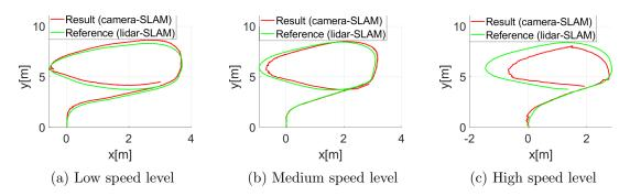
Figure 7.7: Asymmetric circuit - visualisation of estimated path
