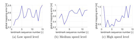
Figure 7.6: Asymmetric circuit - global mapping error
