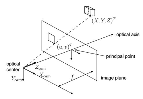
Figure 2.8: Perspective camera model illustration (from [53])
