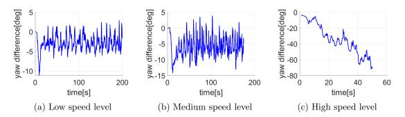
Figure 7.19: Global SLAM - orientation error on the asymmetric circuit
