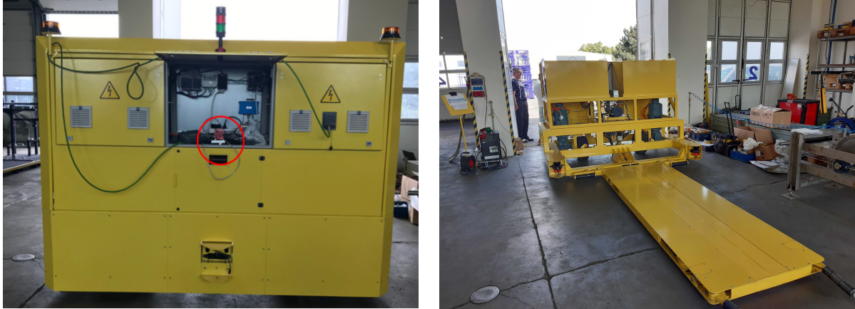
Figure 22: Car-like platform where (left) front image with the radar in red circle (right) Platform from the back
