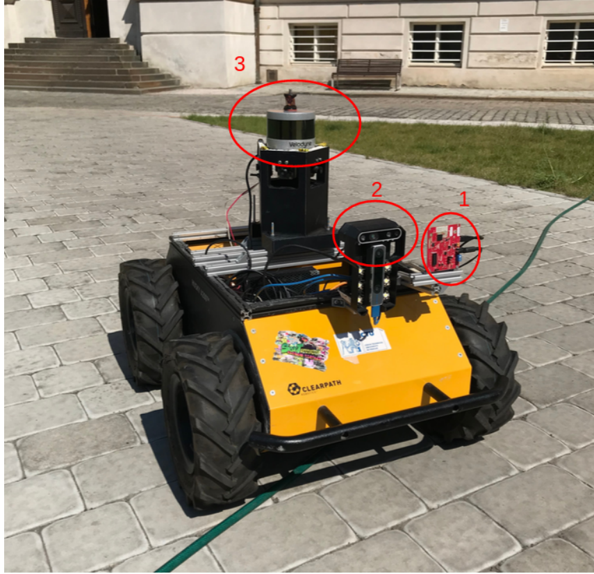
Figure 18: Husky A200 platform equipped with sensors. The red circled sensors are those being used for this experiment as follows: 1) a Texas Instruments IWR1443BOOST 3D radar, 2) an Intel Realsense D415 RGB-D camera, and 3) a Velodyne Puck VLP-16.
