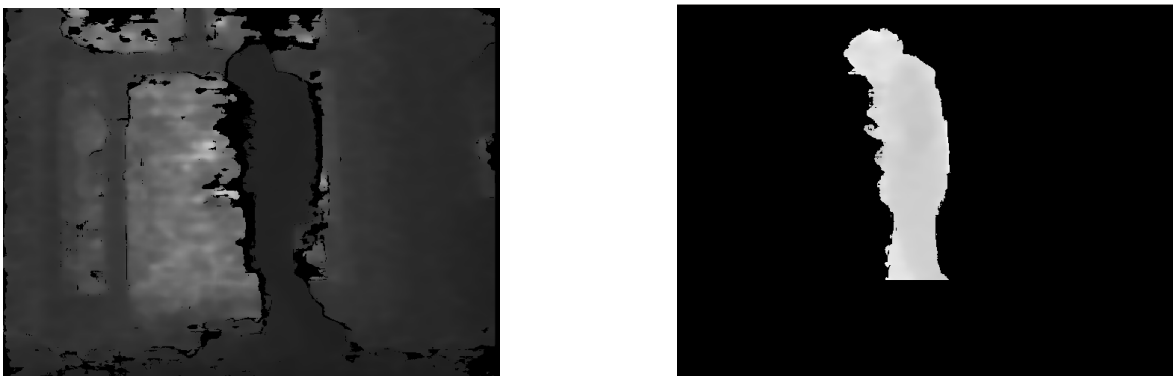
Figure 15: Obtaining ground truth (left) Standard depth image (right) Filtered and clustered person
