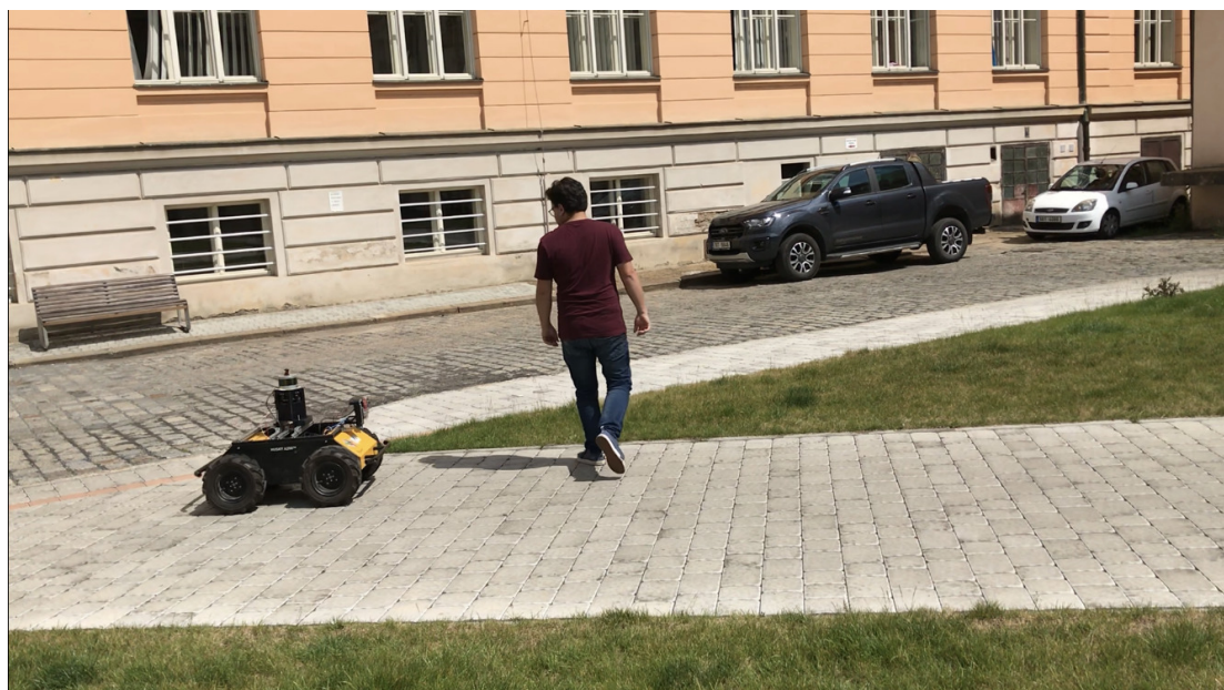
Figure 20: Experiment on a real robot with pedestrian crossing its path during the autonomous navigation.
