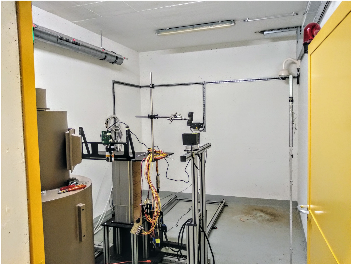
Figure 6.3: A view into the CC60 irradiation room. On the left, a 5-ton “sarcophagus” houses the 10 TBq gamma radiation source. The source is normally stored in the heavily shielded bottom part, and is pneumatically lifted to a height of 1.5 m when irradiation is being performed. A collimator is installed on the front (obscured in this picture) to shape the beam into 30° horizontally by 30° vertically.
