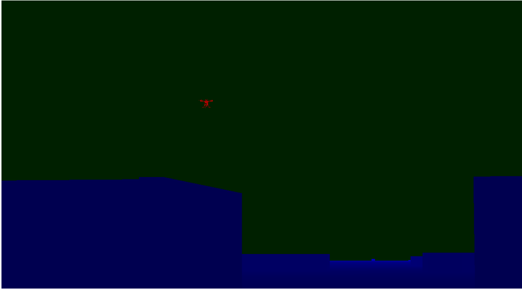
Figure B.8: Detection of a large drone 180 m away from the camera with full HD resolution and 30^\circ FOV. The number of detected pixels is 141.
