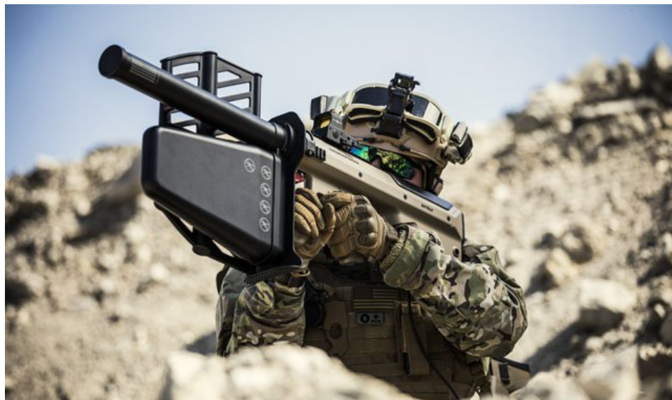
Figure 2.5: DroneDefender Counter-UAS Device, Battelle 7
