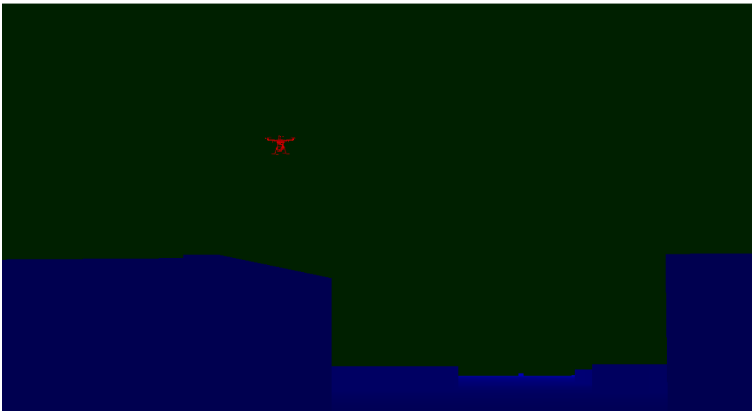
Figure B.7: Detection of a large drone 120 m away from the camera with full HD resolution and 30° FOV. The number of detected pixels is 323.
