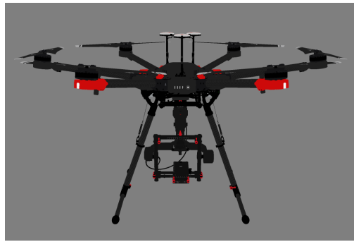
Figure 4.7: DJI Matrice 600 Pro with materials
