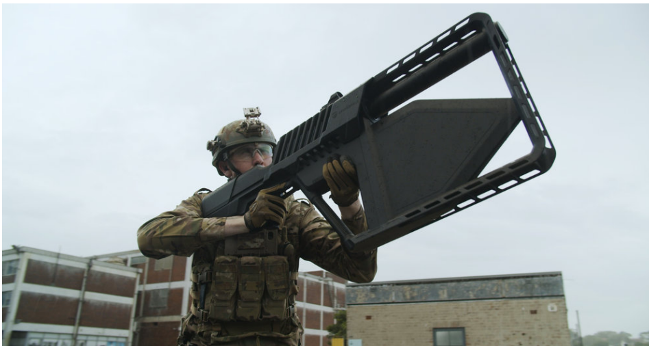
Figure 2.8: DroneGun Tactical, DroneShield 11
