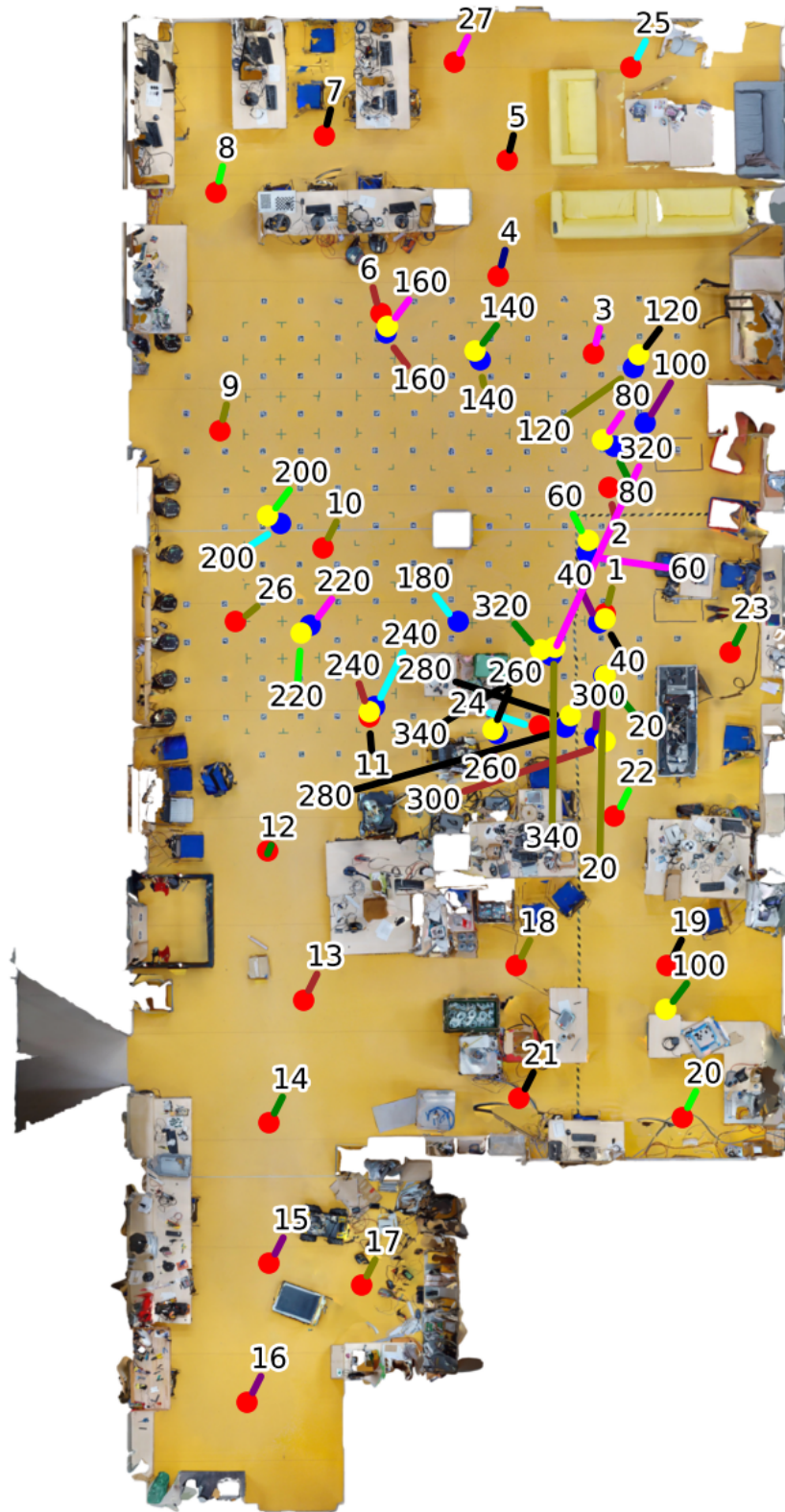
Figure 5.7: View on the floor plan of room B-315. Red dots: sweeps. Blue dots: queries. Yellow dots: estimated query poses. Every 20th HoloLens1 query rendered.
