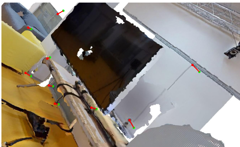
Figure 3.4: Query 94 of HoloLens1 and its reprojections errors. The optimized transformation params were used. The same image on non-optimized parameters is not shown, because the average improvement of reprojection error of a the correspondences is about 2 pixels. Therefore a naked eye can barely tell which image has lower reprojection error. Green points: optimal location of 2D correspondences. Red dots: location of the 3D correspondences (projected onto 2D image plane), under the generic parameters (that aim to work across all queries in the sequence).
