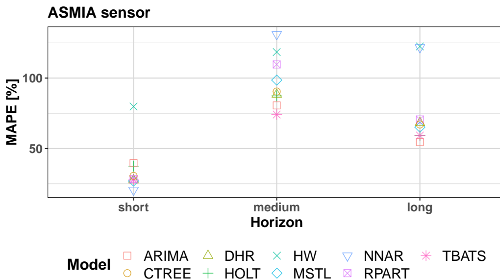
Figure 4.11: Values of the MAPE for all models created from data collected from the ASMIA sensor for 3 different horizons.
