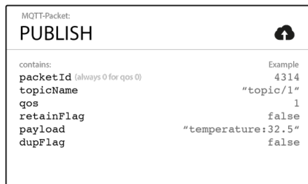
Figure 1.3: MQTT publish packet [19].
