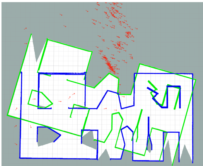
Figure 4.8: The map merging result after 60 iterations with fully explored maze by both UAVs with initial poses on opposite sides of maze.
