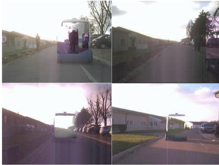
Figure 2.4: The occupancy grid map merging can also be used for estimation of vehicle to vehicle relative pose. With this pose known, we can for example use other vehicles perception to "see" through them. Reprinted from [19, figure 5]
