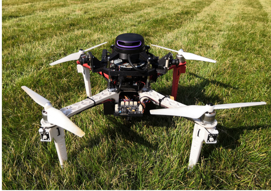
Figure 1.1: F450 quad-copter equipped with 2D Slamtec RPLIDAR A3 360° which was used in this thesis real-world experiments.
