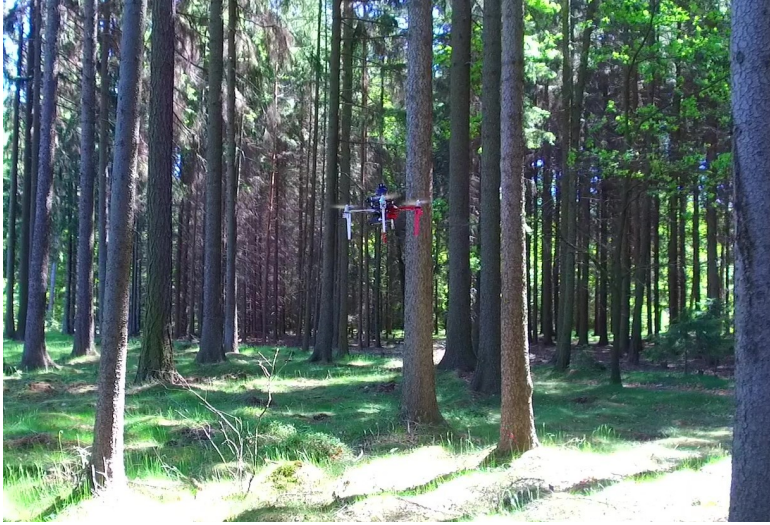
Figure 4.2: F450 equipped with 2D LIDAR and height sensor using HectorSLAM to navigate through a forest.
