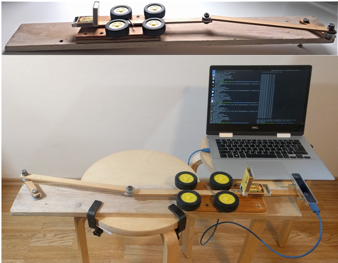
Figure 5.5: The slider-crank measurement device built to perform experiments with Mbientlab MMR sensor and RealSense T265 tracking camera. The device consists of three revolute joints and one sliding joint realized by four wheels. The MMR sensor can be placed in the paper boxes in three different configurations, the camera can be mounted with two screws at the end of the sliding part in three different configurations as well.
