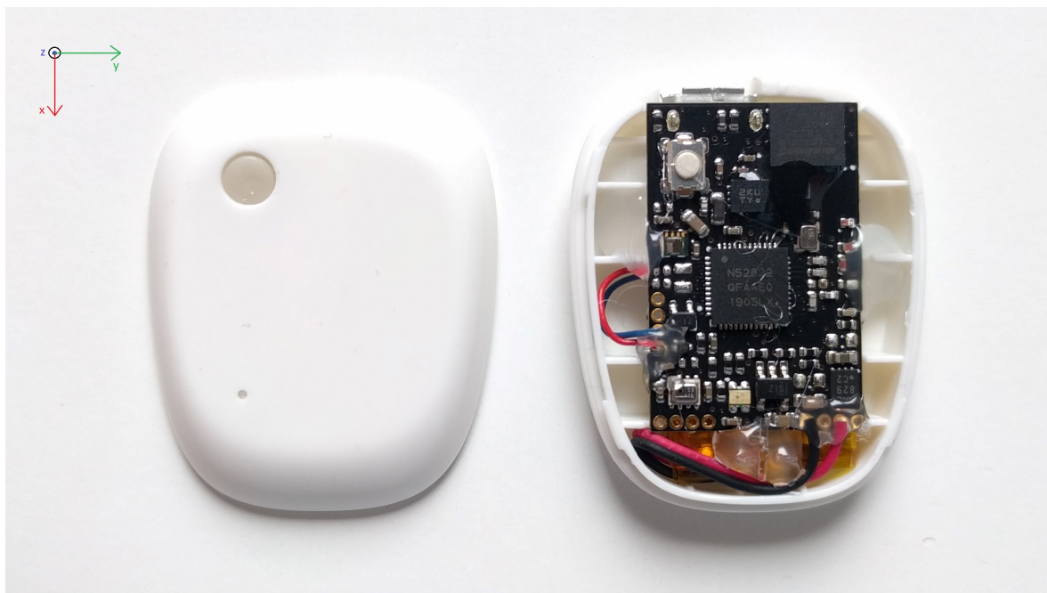
Figure 5.4: The MetaMotionR+ sensor by Mbientlab. The PCB and battery are enclosed in a plastic case (now open). Dimensions 27x27x4 millimeters, weight 6 grams. The orientation of the body coordinate frame is shown (following the RGB-xyz convention).
