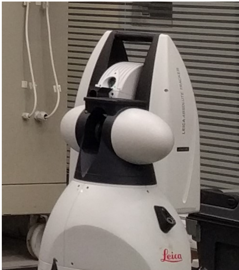
Figure 5.1: The absolute laser trackers AT901 (front) and AT960 (back) by Leica. Dimensions ca. 250x250x500 millimeters, weight 15 kilograms. [37].
