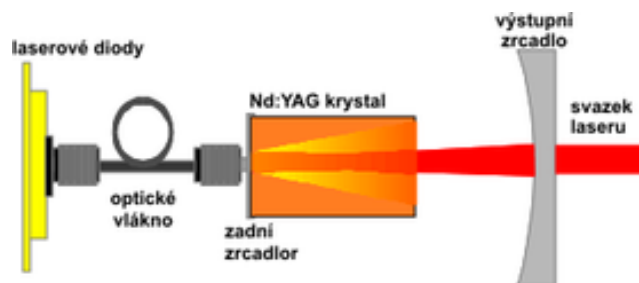
Obr. 9 Princip laseru DPSS [18]
