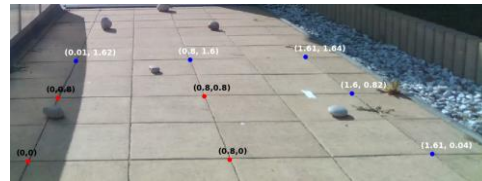
Fig. 5. Using homography to estimate points the location of 3D points. Red points were used for calibration, blue points were estimated by the homography. The error stays within 5 cm.
