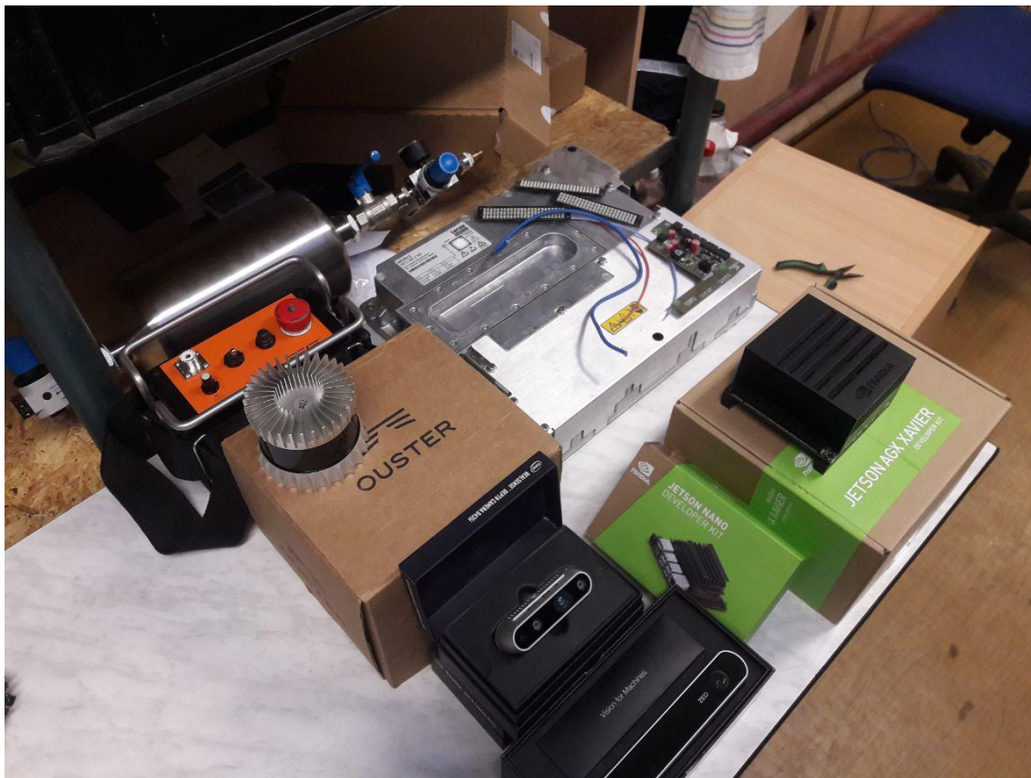
Figure 49: Some of the needed physical technology resources. From bottom clockwise: stereo cameras (Intel Realsense and Stereolabs ZED), LiDAR, Remote Emergency Shutdown, Emergency Brake air reservoir, inverter with electronics, computational units (Nvidia Jetson)
