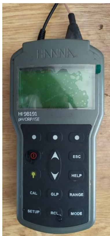
Obr 33 – pH metr HANNA intruments HI 98191
