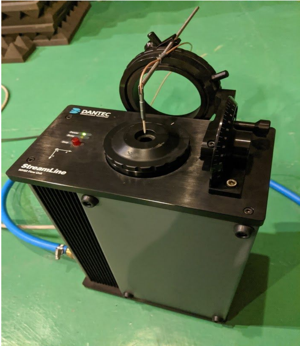
Figure 3-3 Dantec calibrator with dantec hot-wire anemometer probe mounted on it.
