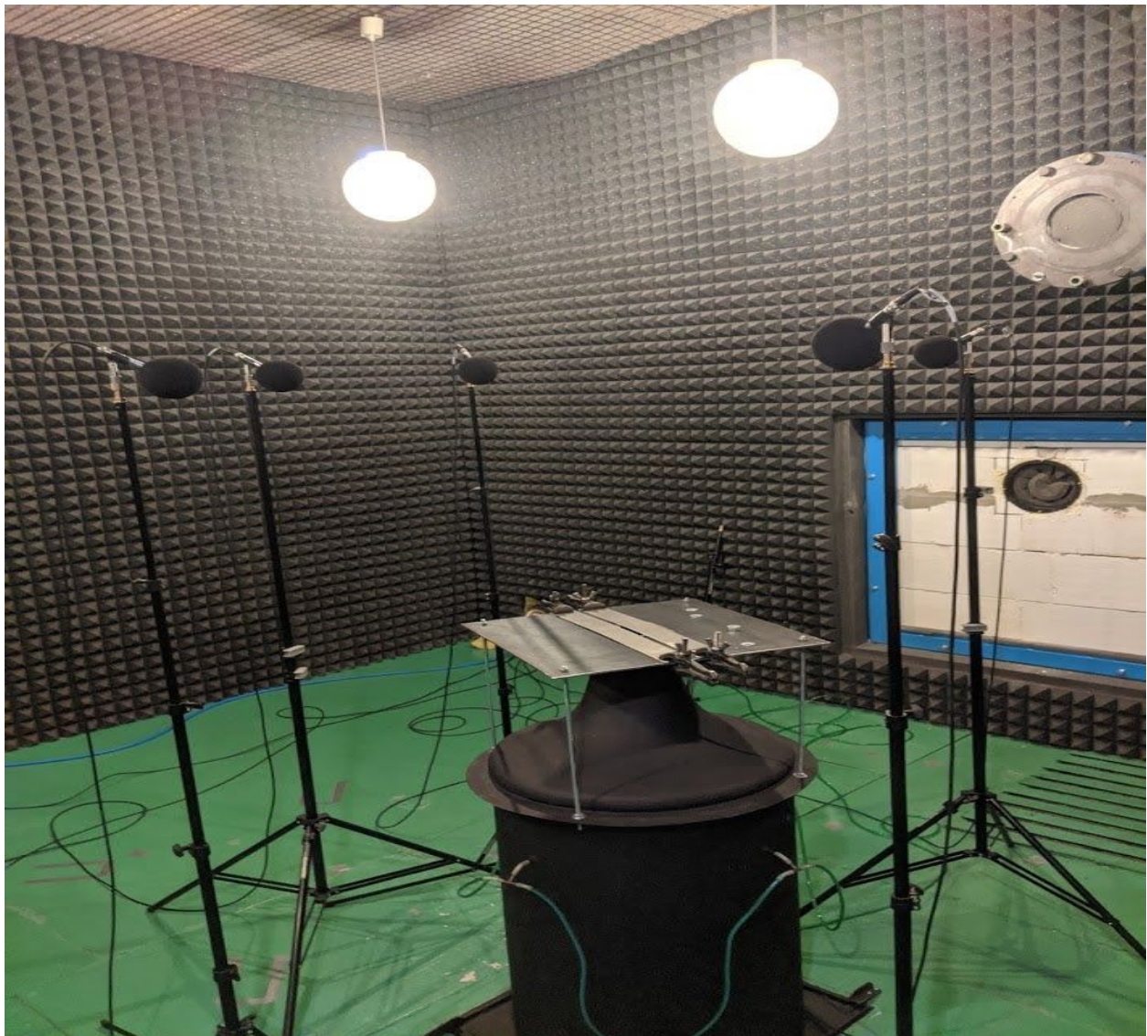
Figure 4-1 Setup of the aerodynamic noise measurements.
