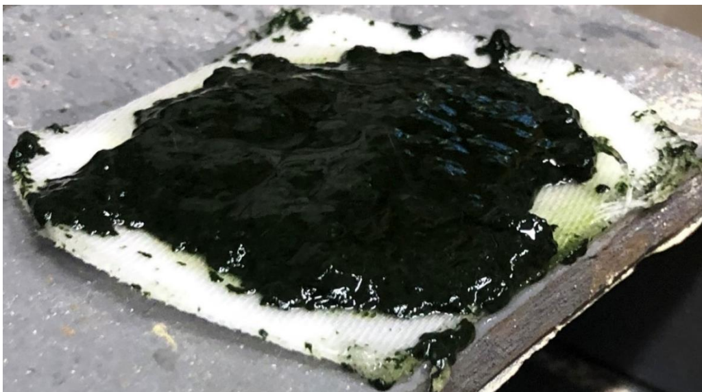
Fig. 22. Membrane surface clogged by flocculated algal cells
