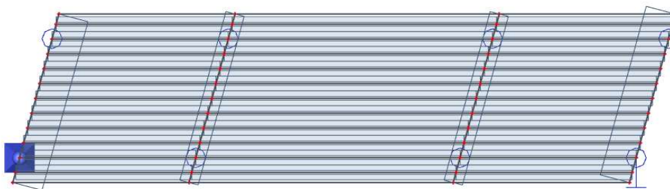
obr. 2.2 Model mostu s šikmostí 75°
