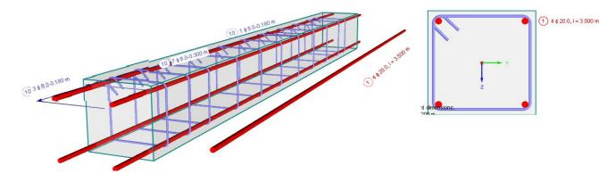
Shear reinforcement for column:
