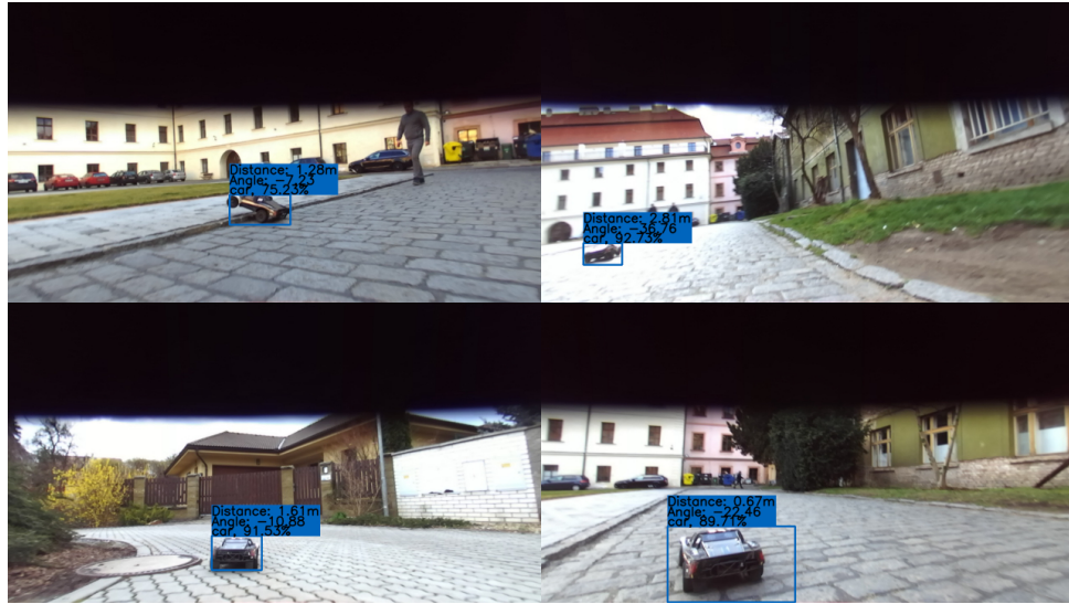
Figure 4.7: Detection bounding boxes, distance, and angle estimation performed on images from the RC car camera. The images are part of the test split of the collected dataset
