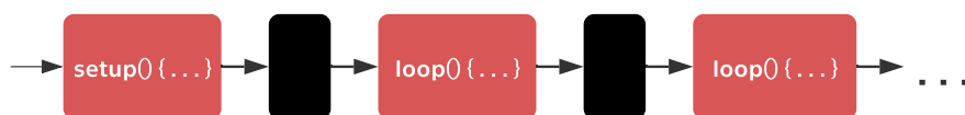
Figure 4.4: Program execution — the setup() and loop() functions are user defined while the black rectangles signify the asynchronous functions and WiFi management
