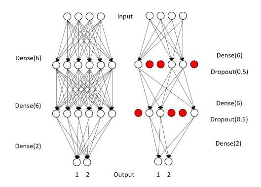
Figure 3.11: Final dense layers with 0.5 droupout. The real network uses Dense(512), Dense(512) and Dense(3) [3].
