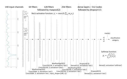
Figure 3.10: Convolutional network workflow [3]
