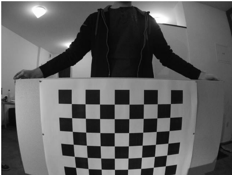
Figure 6.1: An example image from the camera calibration with the calibration pattern present at the bottom of the frame. The pattern appears smaller at the bottom.
