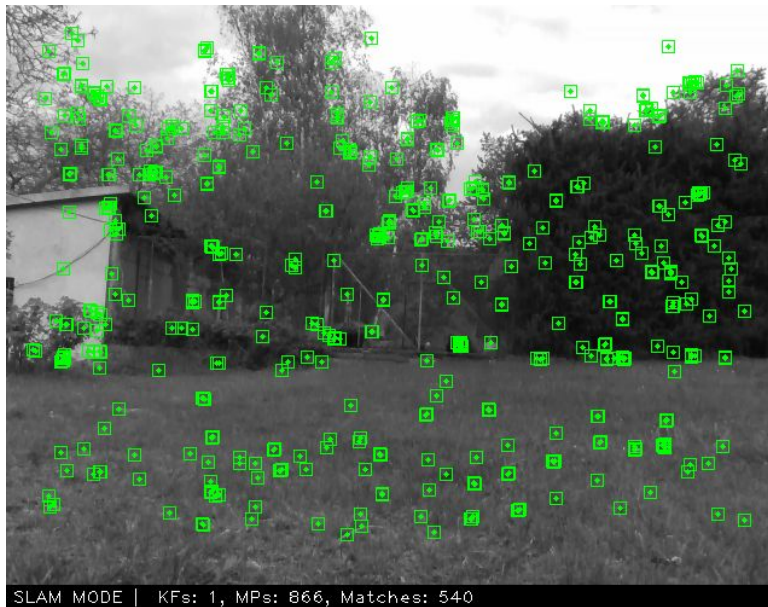
Figure 8.5: An image from the start of the run, most of the the tracked features (green squares) is more than 10 meters away
