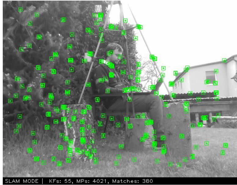
Figure 8.6: Closer objects resulted in localization error of the SLAM method
