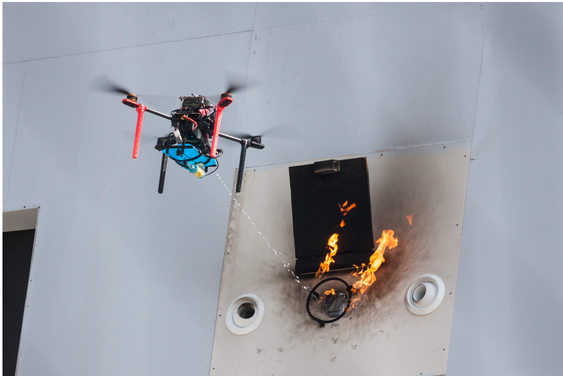
(c) UAV extinguishing an outdoor fire on the facade of the building
