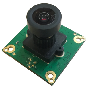
(a) Illustrative photo of the IMX477 4k camera module. Our setup does not use the lenses.
