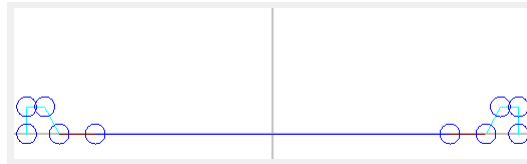
Fig. 11. Example of a track profile (here gray vertical line is the position of the middle curve, circles represent individual vertices, and edge colors corresponds to different material presets)
