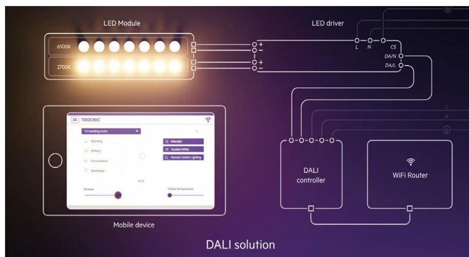
Figure 27. The basic wiring layout of an LED module with DALI [8]
