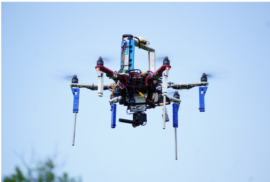
Figure 1: An example of multirotor UAV used in the MRS laboratory.
