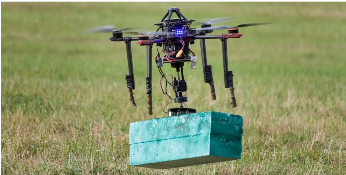
Figure 6: Gripper v1 during an experimental flight in May 2019. Single UAV mode, electronics, and communication were tested.
