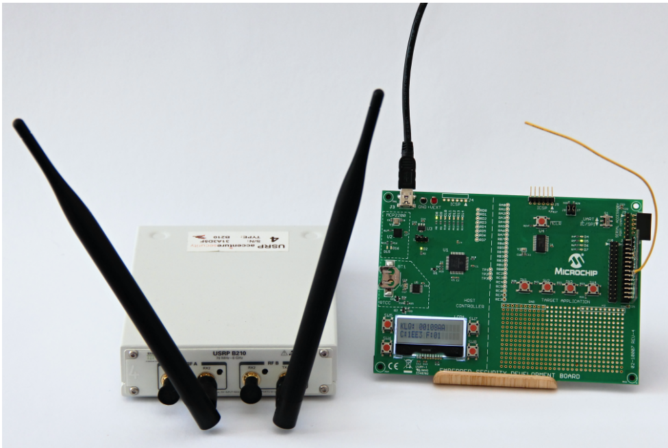
Figure 8.1: Common hardware setup of the demonstration platform
