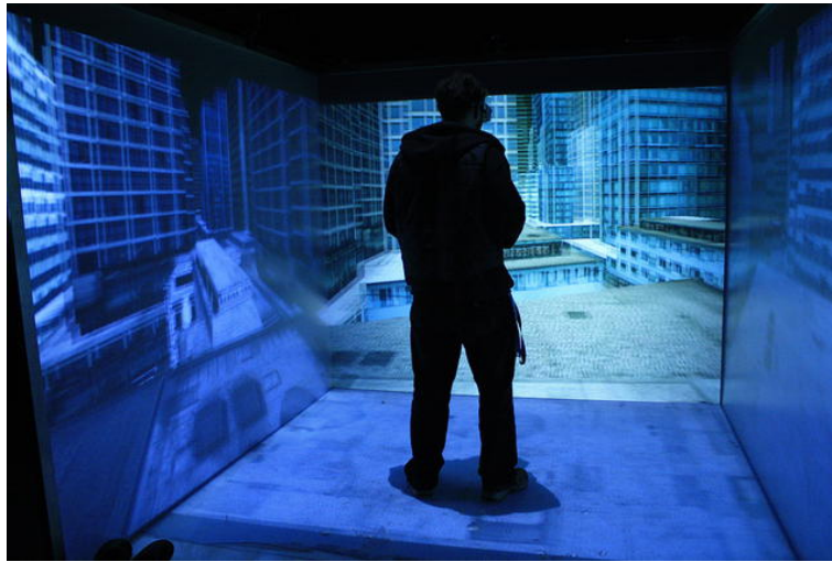
Figure 2.8: Example of a Cave room at Faculty of Electrical Engineering at Czech Technical University in Prague [3]
