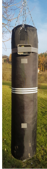
Figure 4.1: Boxing bag used in experiments. Grey marks show the target positions of top and bottom punches. Middle punches were led on the white stripes in the middle of the bag.
