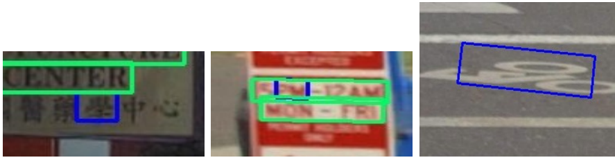
Figure 7.2: Failure cases of our PGT method (blue) - sometimes, very blurred texts, texts in unknown scripts or text-like patterns are recognized as short, common words such as 'on', 'the' or 'in'.
