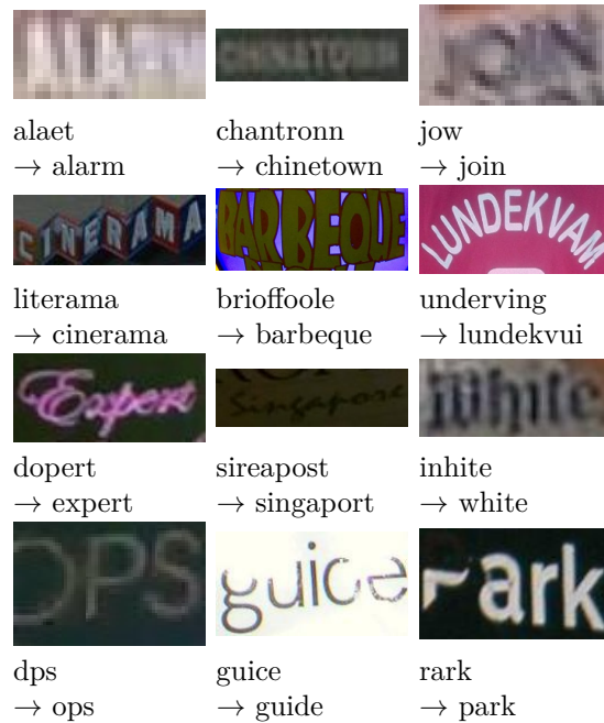
Figure 7.3: Images where the edit distance between the prediction and the ground truth decreased after training with PGT. OCR prediction (first line) and \text{OCR}_{\text{UT}_6+\text{ABC}_3} prediction (second line) are shown below each image. Some common characteristics are blur, occlusion, perspective distortion or artistic fonts.
