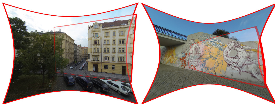
Figure 2.10: Radial-Distortion Homography . The images in each panorama were stitched using the radially-distorted homography estimated by the solvers proposed by Kukelova et al. [45]. This figure is taken from [45].
