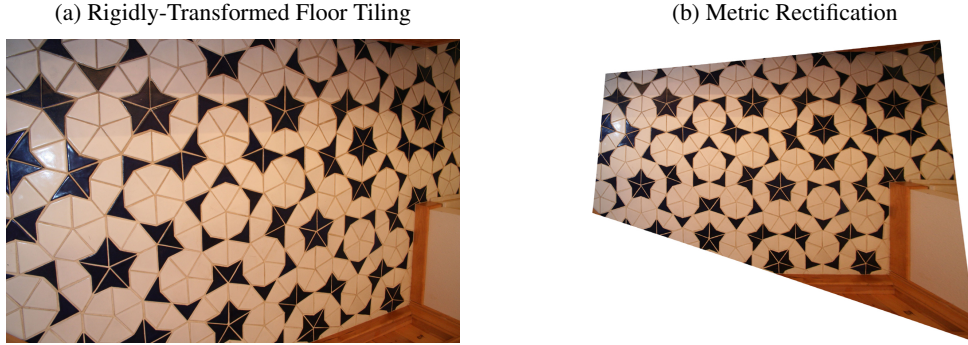
Figure 2.8: Metric Rectification from Rigidly-Transformed Line Segments. (a) Image containing rigidly-transformed line segments. (b) Metric rectification of floor from congruent line segments. Note that the room corner is restored to a right angle in the metric-rectified image.
