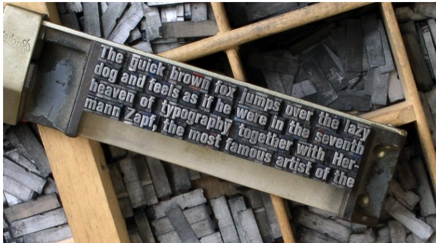
Figure 2.1: An example of Movable-type. Source: [2]
