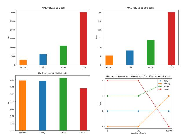
Figure 7: MAE values of different models at different resolutions and the order (lower is better) of the models at different resolutions.
