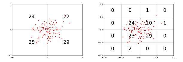
Figure 1: Visualization of the issues of discretization. Cluster of observations on the border of cells.
