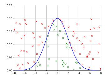
Figure 4: Visualization of rejection sampling using a univariate normal distribution. The green points are accepted and the red ones rejected.
