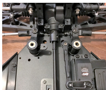
Figure 3.6: Front axle independent steering pivots ready for servo connection
