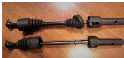
Figure 3.11: Comparison of rear (top) and front (bottom) wheel drive shafts. For the rear axle the former had to be replaced with the latter.
