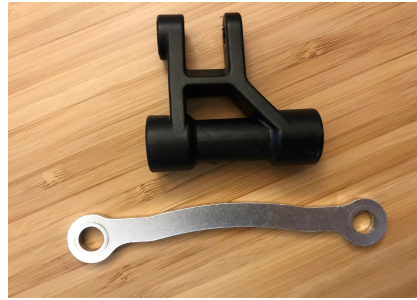
Figure 3.4: Connecting rod and steering pivot from the front axle which are to be replaced in order to allow for independent steering
