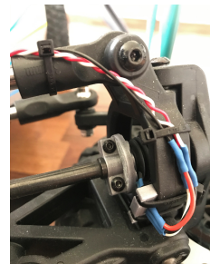
(b) : Installation of the disc and Hall sensor
