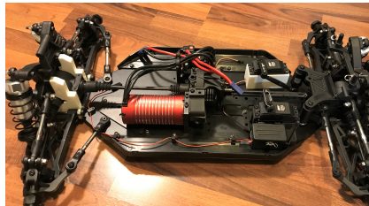
Figure 3.15: With the modified rear axle mounted to the platform the next step is to set up the rear steering links and servos
